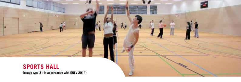
In a sports hall, lighting should be automatically controlled according to requirements, i.e. activated by daylight and by the presence of people. Each section of the hall to be switched independently.
