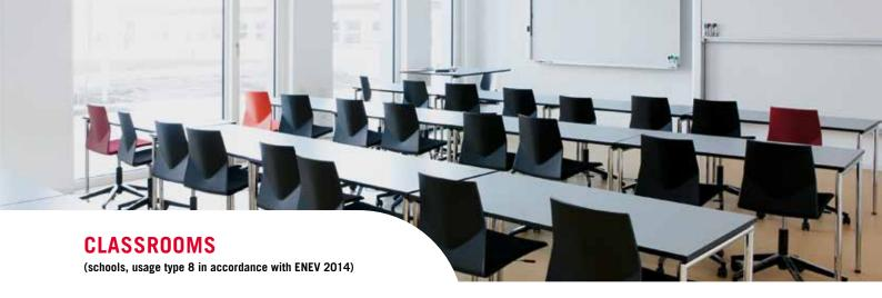
In a classroom, lighting should be automatically regulated to a constant light level according to requirements, i.e. activated by daylight and by the presence of people. The window and wall lighting strips should be switched and controlled independently of each other. The strip lights should be switched on manually via a button while the panel lighting (i.e. for a white/blackboard) is switched separately.
