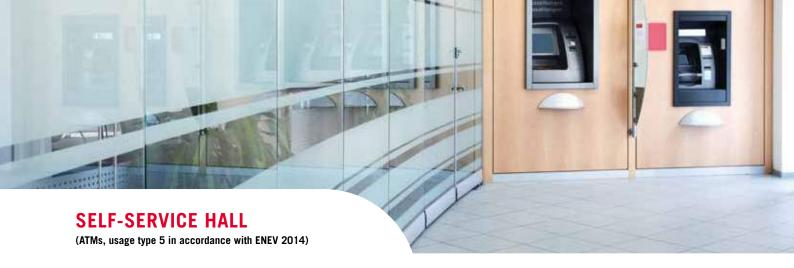
In the self-service area of a bank the lighting should be automatically adjusted according to requirements, i.e. activated by natural light and the presence of people. Outside of business hours there should always be basic lighting of 10%. When a person enters the room, the lighting should be increased to 100%.
