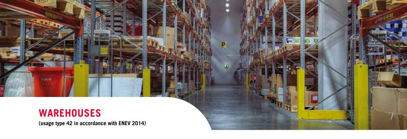
In a high bay warehouse, lighting should be automatically controlled based on demand, i.e. dependent on natural light and the presence of people. The lighting in the individual aisles should then only switch on when each aisle is entered. The main aisle is regarded separately. Orientation lighting of 20% is required.
