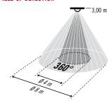
Head-on to detector approx. Ø 4 m Passage area / diagonally to detector approx. Ø 8 m
