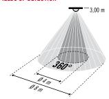
Passage area / diagonally to detector approx. Ø 8 m  $\,$
