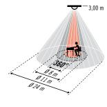
Passage area / diagonally to detector approx. Ø 24 m  $\,$
