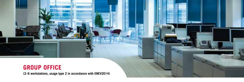
In an open-plan office, lighting should be automatically adjusted according to requirements, i.e. activated by natural light and by the presence of people. Lighting in each work area should be switched on/off individually. Walkways should be regarded as separate from working areas. Each work area is equipped with continuous lighting control and the passage area is equipped with orientation lighting as basic lighting (10%).
