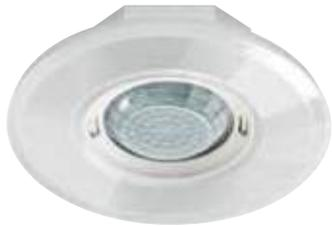
Design presence detector, range approx. 8 meters in diameter, 1 channel, switching, with zero-cross switching optimised for LED lamps, master/slave (parallel connection), low profile design with glass design covers: round, white - variably interchangeable (alternatively: glass, square, black)
