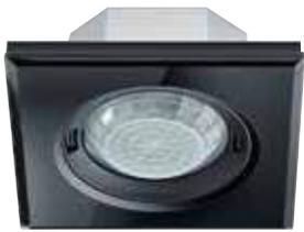
Design presence detector, range approx. 8 meters in diameter, 1 channel, switching, with zero-cross switching optimised for LED lamps, master/slave (parallel connection), low profile design with glass design covers: square, black - variably interchangeable (alternatively: glass, round, white)
