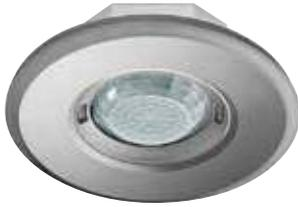
Design motion detector, range approx 8 m in diameter, 1 channel, switching, with zero-cross switching optimised for LED lamps, master/slave (parallel connection), low profile design with plastic design covers: +H1:H2: round, white - variable interchangeable (alternatively: glass, square, black)
