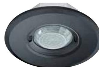
Design presence detector, range approx. 8 meters in diameter, 1 channel, switching, with zero-cross switching optimised for LED lamps, master/slave (parallel connection), low profile design with plastic design covers: round, black - variably interchangeable (alternatively: glass, square, white)
