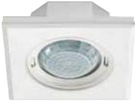
Design presence detector, range approx. 8 meters in diameter, 1 channel, switching, with zero-cross switching optimised for LED lamps, master/slave (parallel connection), low profile design with plastic design covers: square, white - variably interchangeable (alternatively: glass, round, black)
