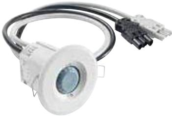
Design motion detector, range approx 8 m in diameter, 1 channel, switching, with zero-cross switching optimised for LED lamps, master/slave (parallel connection), low profile design with plastic design covers: +H1:H2: round, white - variable interchangeable (alternatively: glass, square, black), Wieland GST plug
